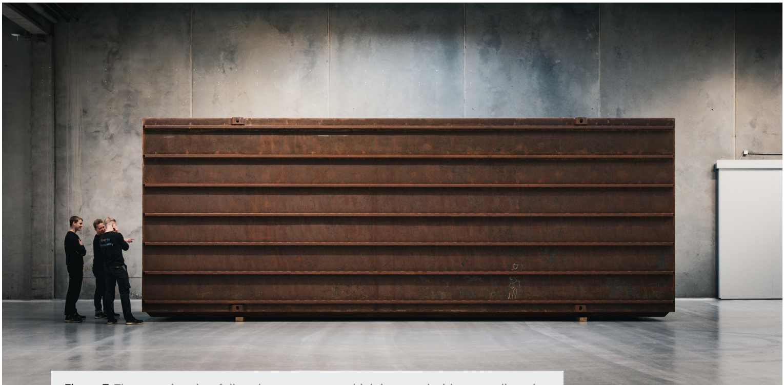
Figure 7. The container is a full scale test reactor, which is tested with non radioactive molten salts. Length: 9 meters, height: 3.6 meters width: 2.5 meters.
